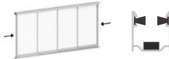
Side vertical profiles surface fitting. Example: rail 4 - tracks
